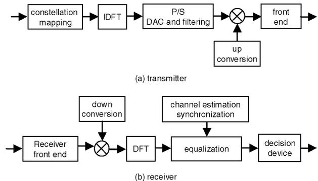
Fig. 1. Block diagram of a general OFDM communication system.
