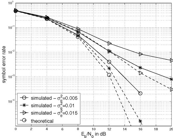
Fig. 2. SER against  $E_b/N_0$  for the AWGN channel. Theoretical results are depicted with dashed lines. Their marker patterns are matched to the corresponding simulation results.
