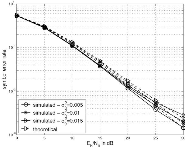
Fig. 3. Theoretical and simulated SER against  $E_b/N_0$  for the frequency selective fading channel. Theoretical results are depicted with dashed lines. Their marker patterns are matched to the corresponding simulation results.
