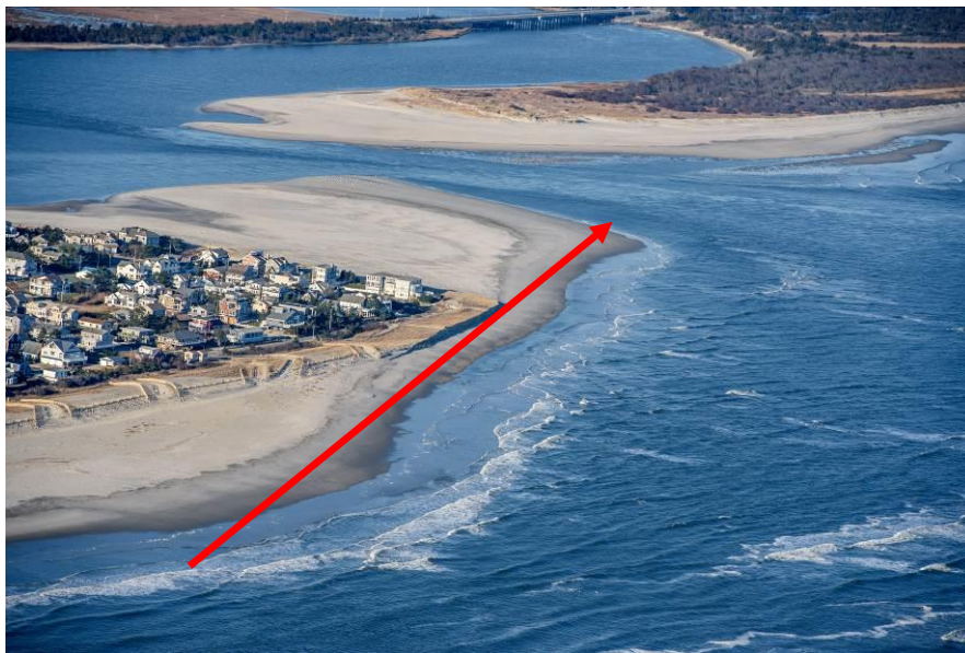
Figure 5. View of Corson's Inlet on December 11, 2018 showing the extent of dune erosion along the same alignment which appeared in September 2017. The impact on the northeast corner municipal dune system is evident. This time there is no subsidiary tidal channel along the beach, but also the offshore bar system lies well seaward as seen in the breaking wave pattern.
