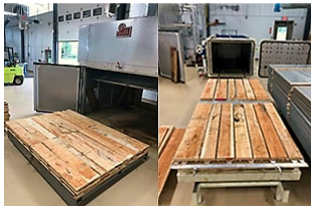
Figure 2: Left, Board sample halves are stacked on stickers prior to processing in the conventional steam kiln; right, board sample halves are stacked on heating platens prior to processing in the vacuum kiln.
