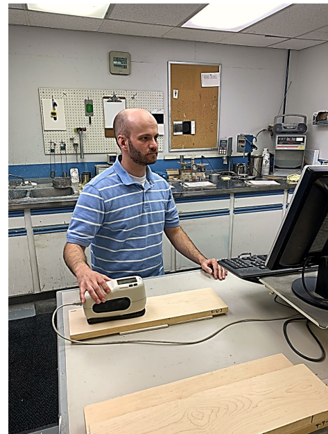
Figure 5. Measurement of a sample board using the Color Master CM2 spectrometer (X-Rite, Inc., Grand Rapids, Michigan, USA) with a D65 light source illumination.
