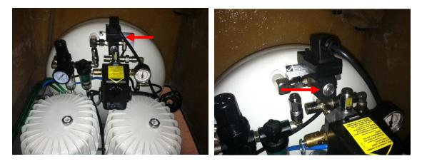
12. Connect the compressor/unit to an electrical outlet to test it. Press the test button on the top of the Auto Drain control module box to test the Auto Drain. You should hear a burst of air; this is the Auto Drain purging the compressor holding tank into the collection bottle, meaning the Auto Drain is functioning properly.
