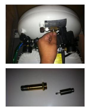
6. Remove any debris or build up and use rubbing alcohol to clean inside the Auto Drain valve.
