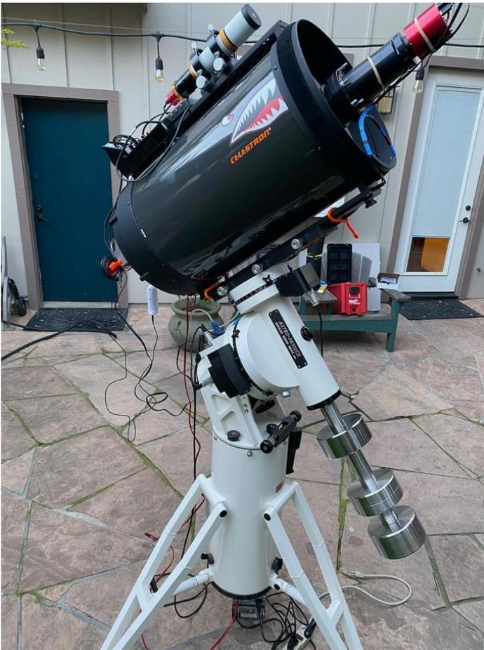
Frank's astrophotography setup, showing, from bottom to top, the white AP1200 tripod and mount with counterweights attached, the large black C14 optical tube assembly with the black Hyperstar unit and red camera attached to its front, and top, the white guide scope and camera attached. (*Frank Seminaro*)
