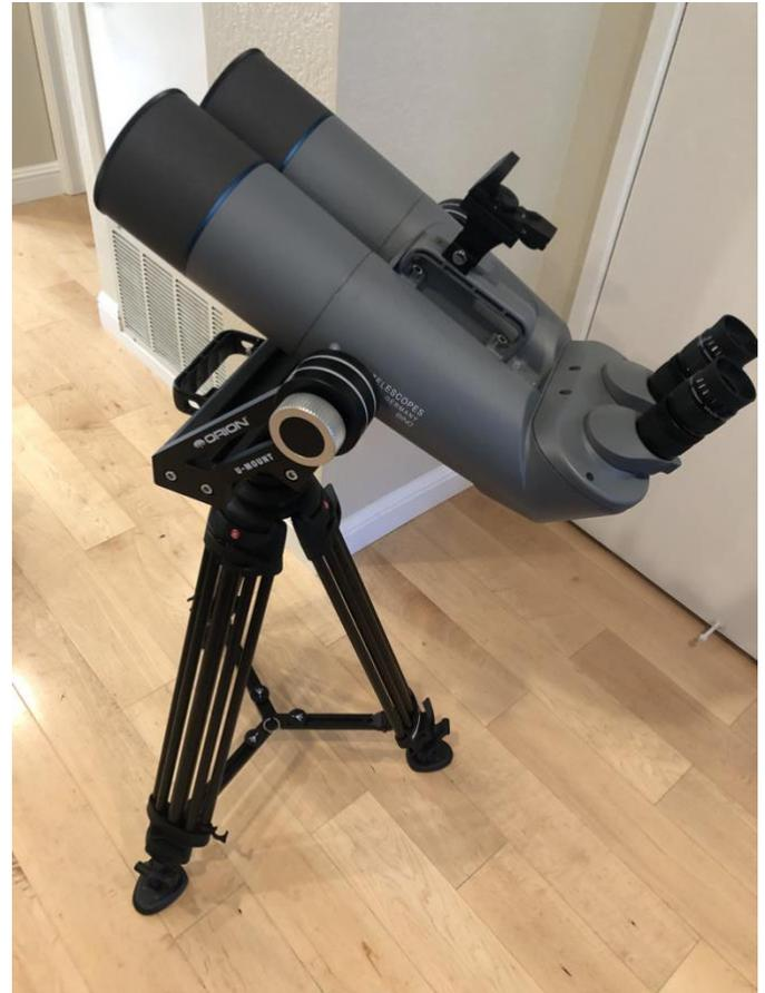
Bill Lockman's APM Binocular telescope mounted on a Manfrotto carbon-fiber tripod with an Orion "U-mount" head. The legs can be extended to raise the telescope to about 5.5 feet. The weight of the tripod and head is about 17 pounds. *(Bill Lockman)*
