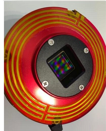
ZWO ASI533MC Pro camera connector end (top) and square sensor (bottom).
