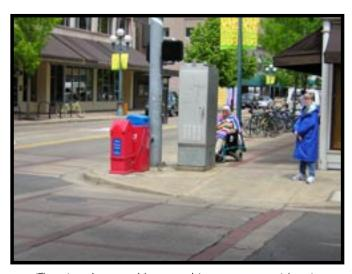
The signal control box at this corner was identified as being a safety problem because it blocks pedestrians from the view of passing motorists.
