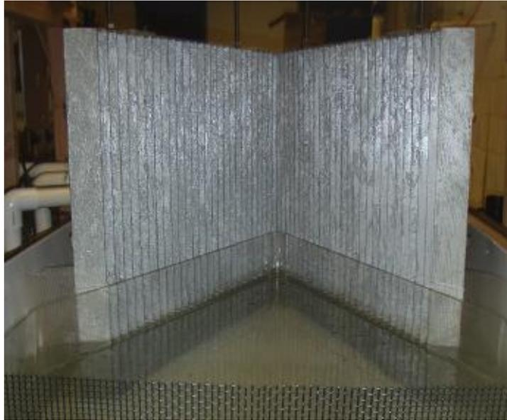
During these trials, an industrial impactor (Martin PKL 150, <http://www.shake-it.com/pkl-interval-imp.shtml>) was used to produce rapid movements of the louver array. The impactor contacted the louver with individual blows, similar to being struck by hammer. We are pleased to report that none of the Rust Bullet coating appeared damaged or was removed by the impactor's operation. Below is a picture of the attached impactor.
