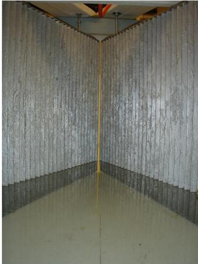
During the freshwater fish swimming experiments, the base of the louver arrays were submerged in freshwater (well water), and the louvers were vibrated with an oscillating industrial vibrator at a low frequency (Martin NTK 25, <http://www.shake-it.com/ntk->
