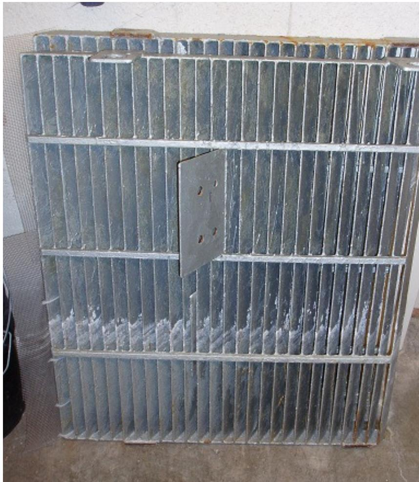
The white layer on the louver array has been made by “hard” water deposits forming on the louver array, just above the water's surface.
