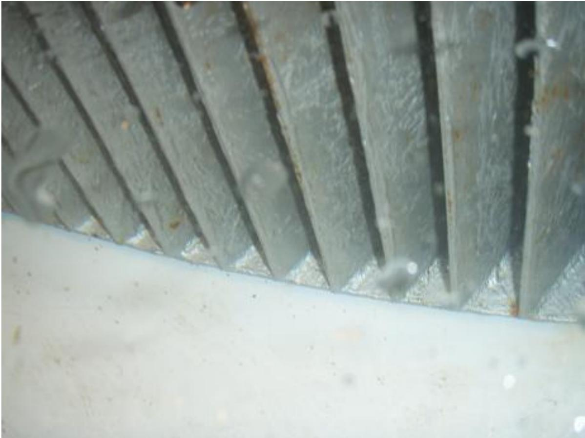
These small patches of rust likely resulted from small gaps being left in the coating when the thick paint was applied, which allowed water to contact the steel.
