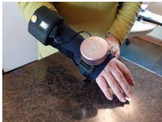
Picture shows a person wearing gyro glove on his right wrist
