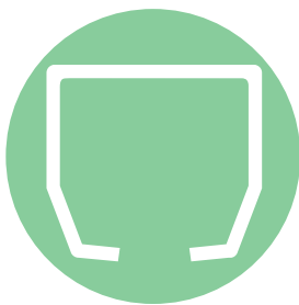
2-degree taper keeps the trolley centered
