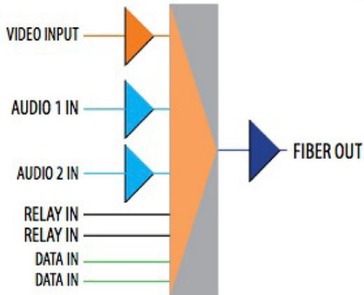
**EMI/RFI Noise and Ground Loops** — Fiber optics are inherently immune to all kinds of electromagnetic interference (EMI) and radio frequency interference (RFI). Also, because a tactical fiber optic cable contains no electrical conductors, it cannot contribute to ground loops. All copper cables are susceptible to both EMI and RFI. This can be limited with cable shielding, but shielding adds to bulk and weight. Also, the cables' metallic conductors and shields can contribute to ground loops.
