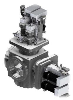
The SLT-600 slit system is designed for UHV and can be used for apertures from 25 mm x 25 mm all the way up to 100 mm x 100 mm. Blades are actuated independently by 4 actuators mounted on the slit body. This slit system was designed to be robust and easily serviceable. ADC draws from an array of standard components to rapidly develop a reliable solution to each beamline's needs.
