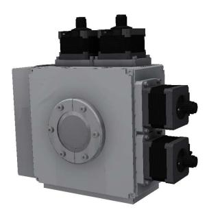
These high-precision slits systems consist of four blades that are housed in an aluminum body. These slits use standard micro-stepped stepper motors that can be controlled with a wide array of controllers/drivers available on the market. The design incorporates mechanical limit switches.
