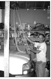
Using hydraulic jacks Vince dropped the battery pack onto a low slung creeper with castors and then hoisted the front of the truck up using the pictured bumper attachment. The truck raised from the front providing clearance to roll the pack out to the side.
