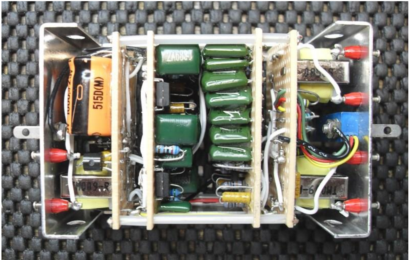
Figure 13: The Assembled Audio Module in Minibox Enclosure
