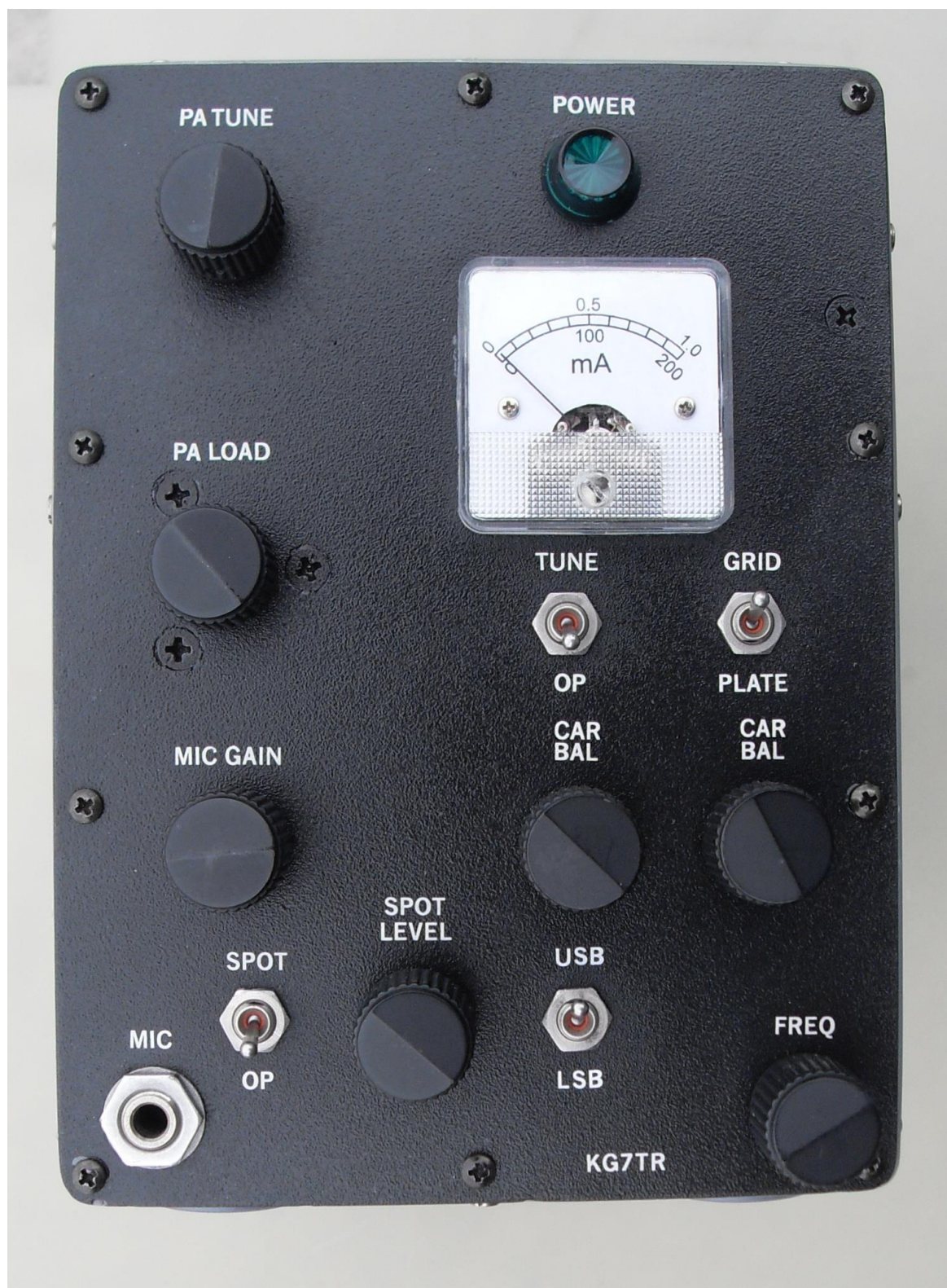
Figure 7: Front Panel. Meter scale is home made using computer drawing program.
