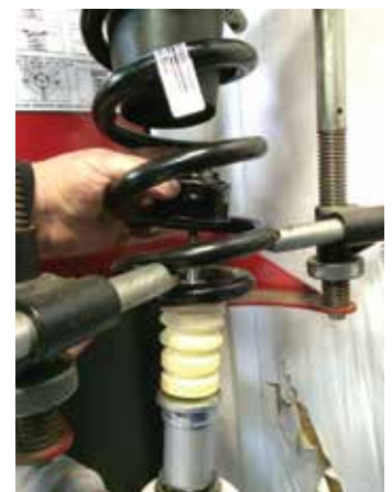
Installing the factory spring & Inner bump stop cup to the new McGaughy's strut.
