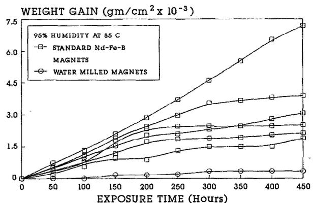
FIG. 5. Weight gain of Nd-Fe-B magnets made from water milled and gas passivated powder during exposure to humid atmosphere.
