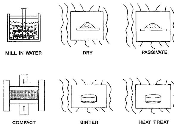
FIG. 1. Schematic of water milling and gas passivation process for the production of sintered magnets.
