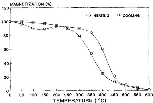
FIG. 6. Magnetization vs temperature of Nd-Fe-B-C magnets produced from water milled and gas passivated powder.
