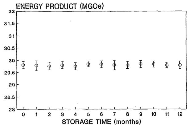
FIG. 4. Maximum energy product of magnets made from water milled and gas passivated powder which had been stored in laboratory air environment.
