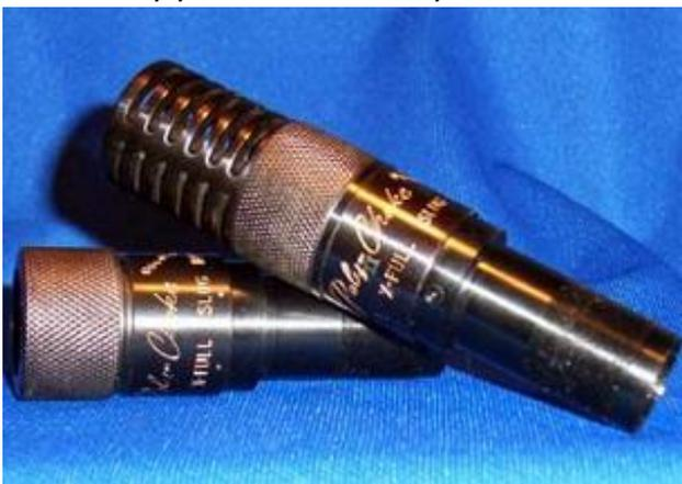
This system functions by manner of a collet which can be adjusted on the fly by twisting the outer sleeve, which is marked for the various amounts of choke. Some models came with a compensator to, purportedly, reduce recoil, most did not. Like the earlier Cutts unit, these become a permanent installation on the barrel. They don't add nearly as much weight as the Cutts, and don't change the handling characteristics or sight line as the Cutts unit does.
