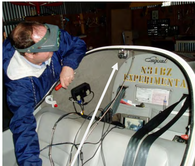
The power inverter was used during ground test only. Note camera to record stick movements.
