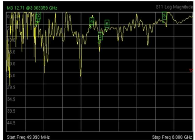
Fig.7: Measured return loss for the first antenna at 3 GHz
