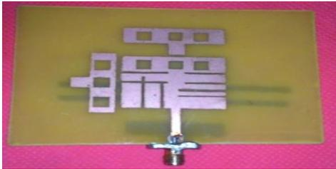
Fig.5: Body Phased Array Antenna showing top plane
