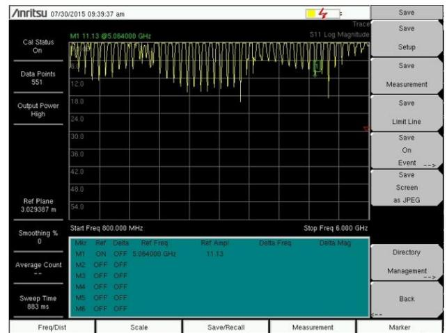
Fig.9: Measured return loss for the second antenna at 5 GHz
