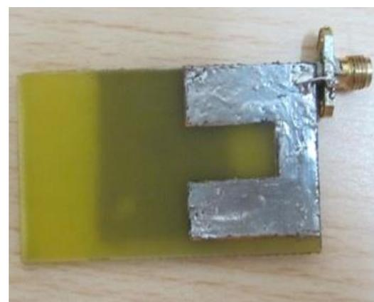
Fig.2: Body Patch Antenna showing bottom plane
