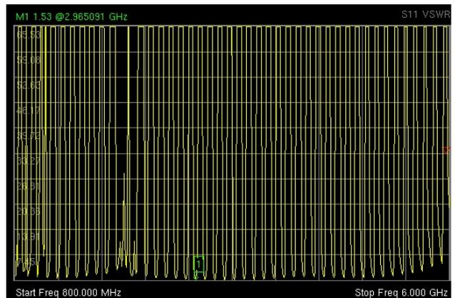
Fig.8 Measured VSWR for the VSWR antenna at 3 GHz
