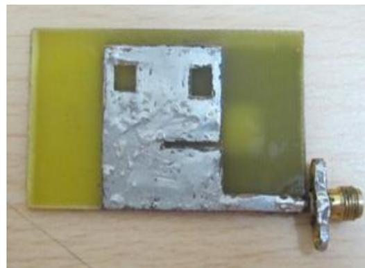
Fig.1: Body Patch Antenna showing top plane
