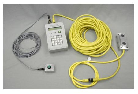
where m is the ram mass, and v is the impact velocity. The proximity switches are mounted directly on the side of the hammer in a pre-machined port. All Berminghammer hammers manufactured since 1990 are equipped with such ports.
