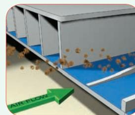
is ground-breaking. Each layer is only 0.08 inches apart, with alternating charges, which makes for a stronger, more
