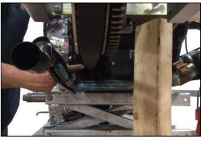
Step 21 Install the Top Mount Assembly, using two 3/8"-16 x 1" Bolts (part #1252), two 3/8" Flat Washers (part #1256), two ½"-13 x 2 ½" Bolts (part #1266), two ½" Lock Washers (part #1262), two Top Mount Plates (part #1268), two 7/8" Top Mount Spacers (part #1270) and one Top Mount Cross Shaft (part #1272)
