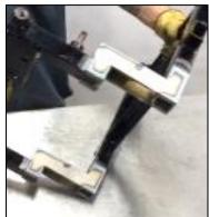
Step 6 Install two bearings (from original trike) into the Swing Arm (part #1244)
