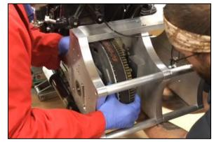
Step 17 Install two stock belt adjusting screws into the front side of the Adjustable Swing Arm Bracket (part #1250)
