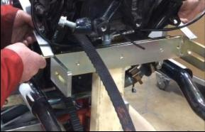
Step 14 Loosely install one Top Mount Hanger (part #1258) using one ½"-13 x 1 ½" Bolt (part #1260) and one ½" Lock Washer (part #1262)
