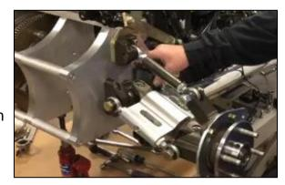
Step 46 Take measurements in four different places around the Brake Caliper Mount (part #1320) from the outside of the Main Assembly (part #1264) to the outside of the Brake Caliper Mount (part #1320). Adjust the Top Support/Adjusting Tubes (part #1306) in order to get equal measurements and square
