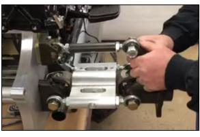
Step 42 Double check the vertical movement of the entire outer assembly
