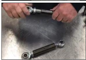
Step 36 Install the Top Support/Adjusting Tube
