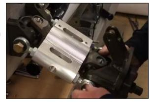
Step 40 Install the bottom Spherical Bearing of the Top Support/Adjusting Tube into the slot on the top of the Outside Carrier (part #1314), using a 5/8"-18 x 2 1/4" Bolt (part #1316), two Spherical Bearing Seals (part #1298) one on either side of the Spherical Bearing and one 5/8" Nylock Nut (part #1318)
