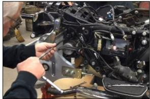
Step 27 Install one Support Bar (part #1284), using one stock 3/8"-16 x 1 ¼" bolt and one stock 3/8" flat washer for the top hole and one 3/8"-16 x 1 ¼" Bolt (part #1286), one 3/8" Flat Washer (part #1256) and one 3/8" Nylock Nut (part #1288) for the bottom mounting hole. Make sure the brake line is **below** the Support Bar
