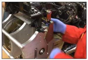
Step 22 Install two 7/16"-14 x 1 ¼" Swing Arm/Main Bolts (part #1274), two 7/16" Lock Washers (part #1276) and two 7/16" Flat Washers (part #1278) to lock Swing Arm and Main Assembly in place
