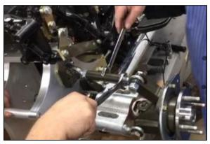
Step 48 Install one Bottom Shock Mount (part #1328), using two 3/8"-16 x 1" Bolts (part #1252) and two 3/8" Lock Washers (part #1254)
