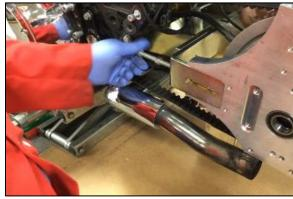
Step 18 Take measurements on both sides of the assembly from the machined edge on the Main Assembly (part #1264) to the center of the transmission cross shaft. Adjust the belt adjusting screws to make the Main Assembly (part #1264) square to the chassis of trike There should be about ½" of play on the Pulley
