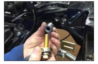
Make sure extra hole is closest to the bottom bearing Repeat Step 14 on opposite side of trike
