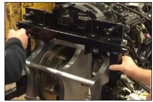
Step 49 Loosely mount the rear body mount frame, using the stock 9/16" hardware
