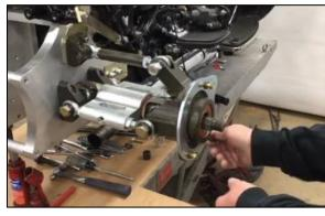
Step 43 Install one Brake Caliper Mount (part #1320) using four 3/8"-16 x ¾" Bolts (part #1322) and four 3/8" Lock Washers (part #1254)
