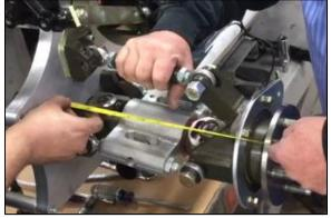
Step 47 Tighten Spherical Bearing Nuts and double check measurements
