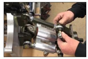
Step 41 Torque all three of the 5/8"-18 x 1 ½" Bolts you've just installed to 80 pounds each
