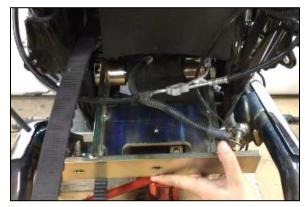
Step 9 Install 1" Spacer (part #1246) onto Swing Arm using a ¼-20 x 2" Bolt (part #1248) to stabilize brake lines
