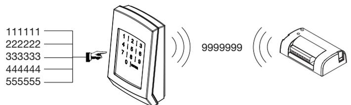
In this example, the “Father” code 999999 is matched to various “Child” codes (111111/222222/etc.). In this way, new Child codes can be included at any moment by acting directly on BE.TOUCH, without having access to the receiver.
