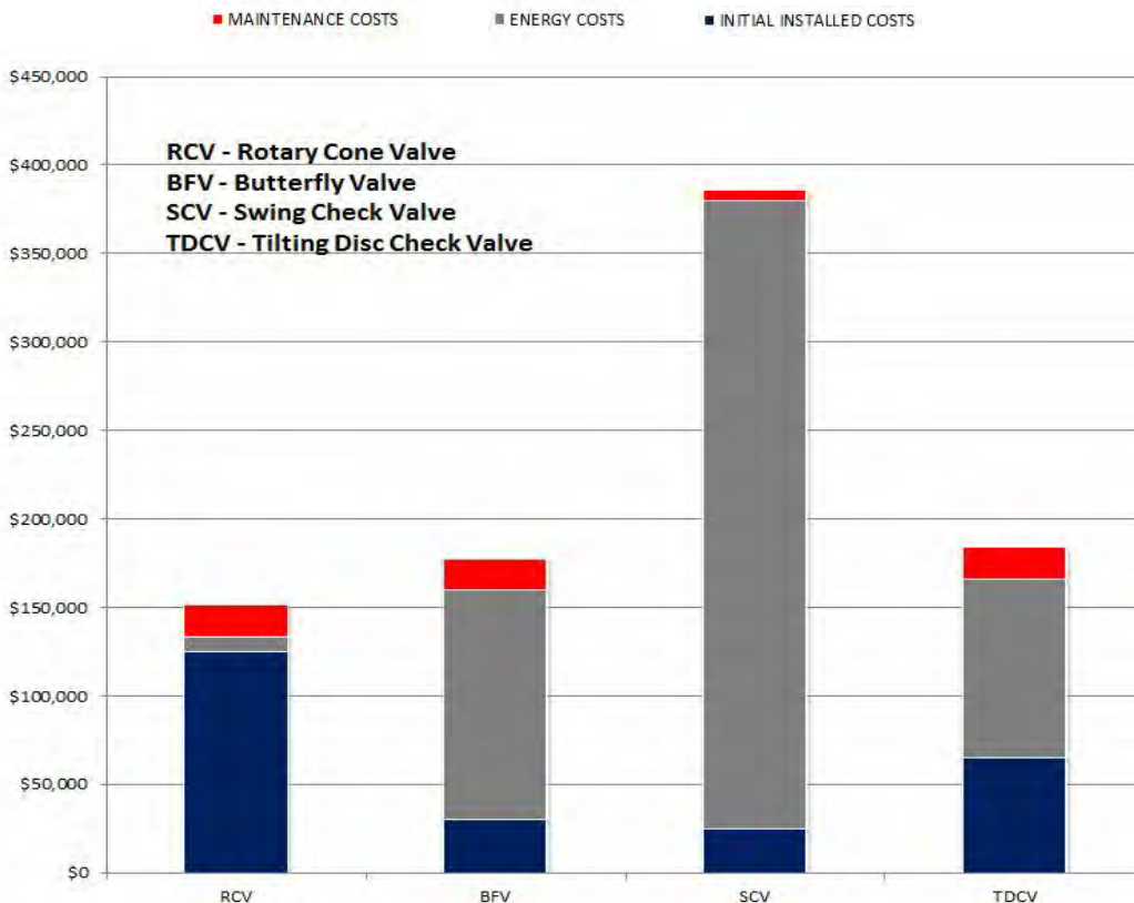
The table depicts estimated annual power costs associated with various types of pump discharge/control valve types. All values are based on $0.12/(kWh), continuous pumping operation (8,760 [hours/year]) at 80% overall pumping efficiency with a discharge velocity of 16 [ft/sec].
