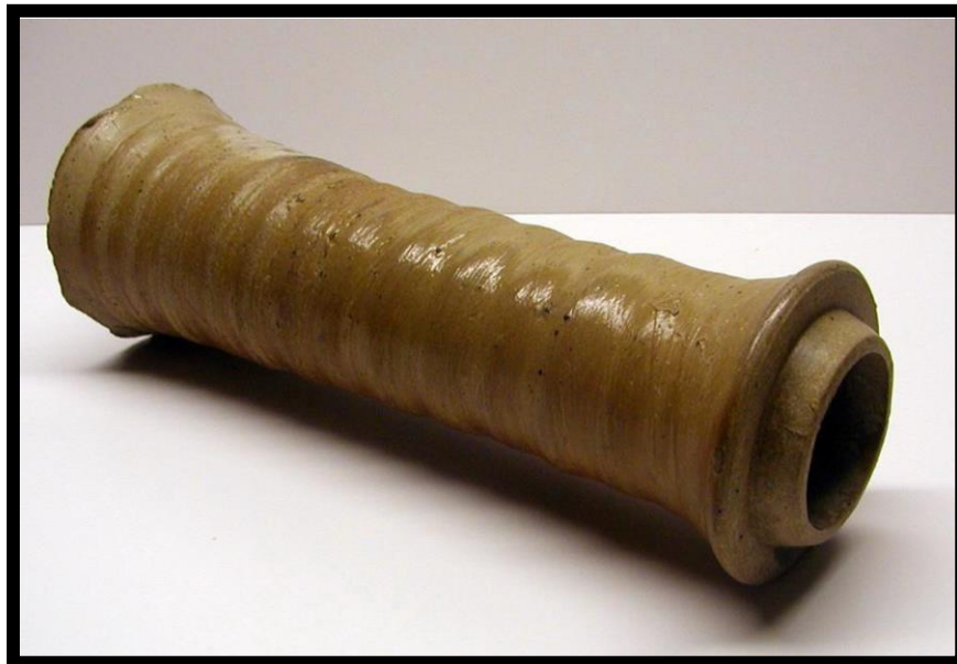
FIGURE 81: Sewer tile drain end cap and standard drain tile pipe section. Approx 18" L, 6" W.
