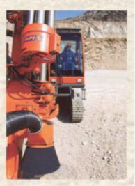
The TITON 500 is a new member in the Sandvik BPI range of DTH drilling rigs. It has been designed to meet the most versatile requirements of mining and quarrying applications and is best suited for 105 - 152 mm hole sizes. Transportability and high compressor output makes it a flexible tool for any quarry, mine or contractor with high productivity requirements and flexible drilling needs.
