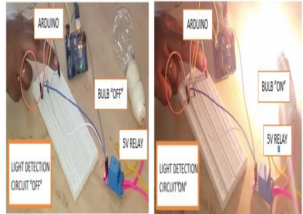
(a) (b) Fig.4 Light detection circuit
