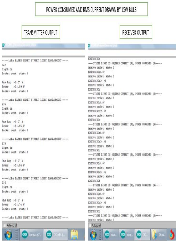
Fig.10- Serial monitor output showing RMS current and power consumed at transmitter and at receiver
