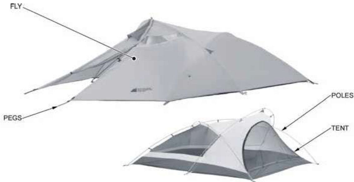
Figure 1 Sample Tent with Labelled Parts (No Guy Lines)
