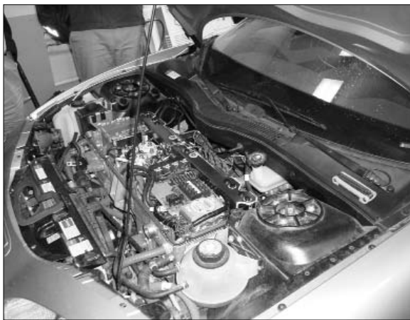
Under the hood of the Penn State EV-1, hybridized with hydrogen.
