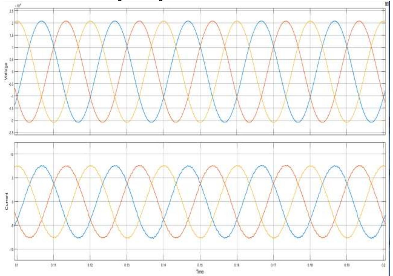
Fig. 8. Voltage and current waveforms at PCC
