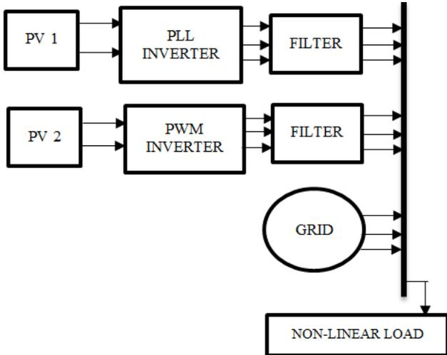
Fig. 9. Block diagram of non-linear connected grid system
