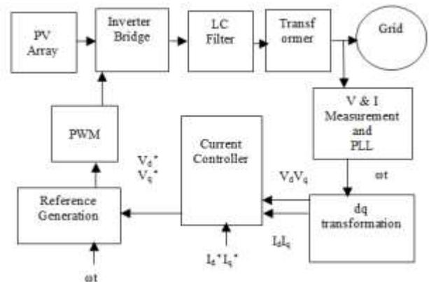
Fig. 3. Block diagram of PLL control for inverter
