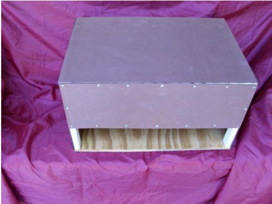
Cabinet with "hardboard" installed, viewed from back
