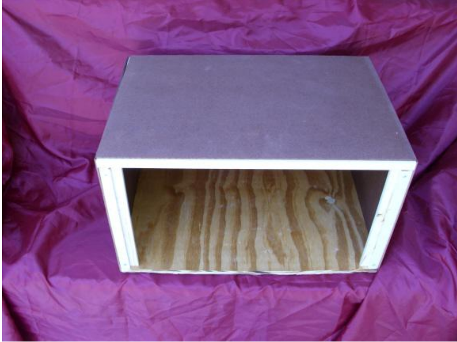
Cabinet with "hardboard" installed, viewed from front
