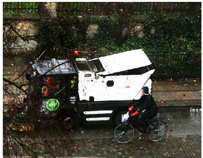
Sweepers in Copenhagen are designed specifically for bicycle facilities and can sweep or clear snow (Photo: Copenhagenize)
