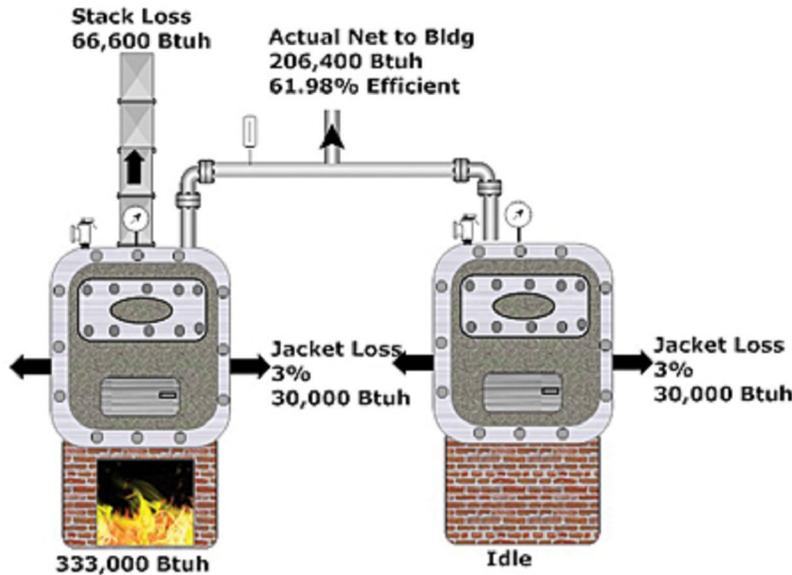
For years we have designed boiler rooms consisting of two oversized boilers with fully modulating burners. The idea was that the boilers could “loaf” along at low fire because we were told they were more efficient at low fire. I think it is time to rethink that strategy.
