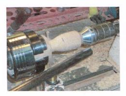
Once you have parted off the bottom, a short piece of 1/8" dowel is glued in the perch hole and you are done. Now is the time for finishing and gluing the roof to the bottom. For a nice touch, Craft Supplies has a number of birds from which to choose that can be mounted on the perch.
