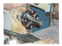
Mount your work on the Jam chuck. This is why we left the hole in the top 1" and left a 1/4" shoulder on the bottom. You can now complete the bottom however you choose. In this case, the original blank was long enough to turn a base.
