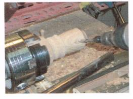
Hollow out the inside. Do not enlarge the first 1/8 to 3/16 of the bored hole. The walls should be 1/16"-1/8" thick. The hollowing should be just past the perch hole and leave about a  $\frac{1}{4}$ " shoulder on the 1" bored hole. Mark the outside 1  $\frac{3}{4}$ " (the bottom of the 1"
