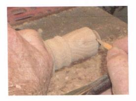
Drill the Entrance and perch holes. The Perch hole is 1/8" and the entrance hole is approximately 7/32". The perch hole should be directly under the entrance hole. The holes will be positioned more accurately if they are started with a hole made by an awl or center punch.
