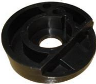
Part Name: Brush Socket Part No.: HEL2-3400061 Remark: Assembled between Steering Wheel and Steering Column. Horn Wire is assembled on it
