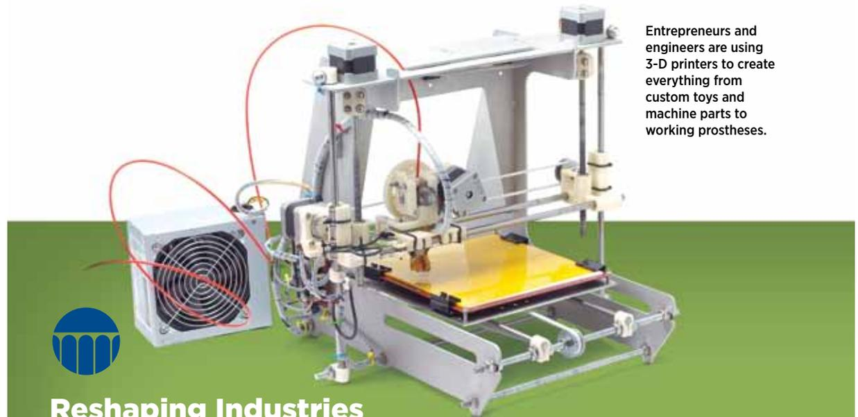
Entrepreneurs and engineers are using 3-D printers to create everything from custom toys and machine parts to working prostheses.
