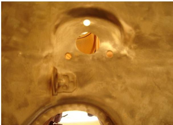
Step 2. Before attaching the panels, check the chassis for cracks, especially around all production welds and where two or more panels come together, and repair any cracks or rust. Below you see how the chassis has been stressed by the sway bar and has cracked by the top bolt hole. This crack and the holes should be welded and ground down as new holes will be drilled for the new stiffening panels.
