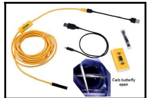
Figure 34 Endoscope showing carb butterfly open
