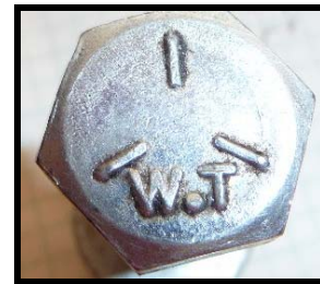
Figure D – Typical Bolt Head Marking
