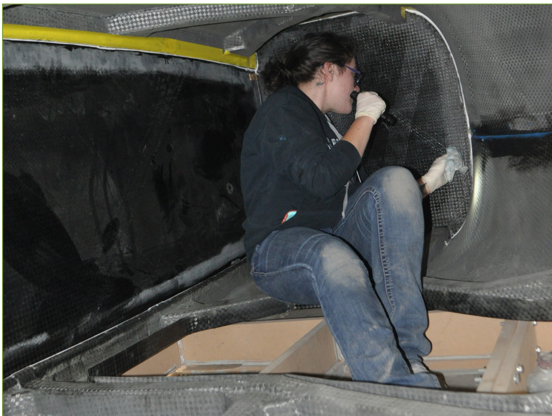
Airplane fuselage halves being bonded together at Composite Approach in Redmond.
