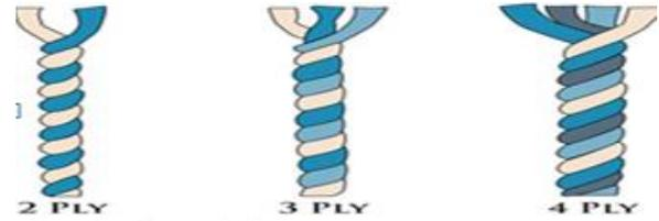
Figure 2. Different twist level yarn
