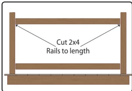
**STEP #1** - Measure distance between posts and cut 2x4s to create top and bottom rails.
