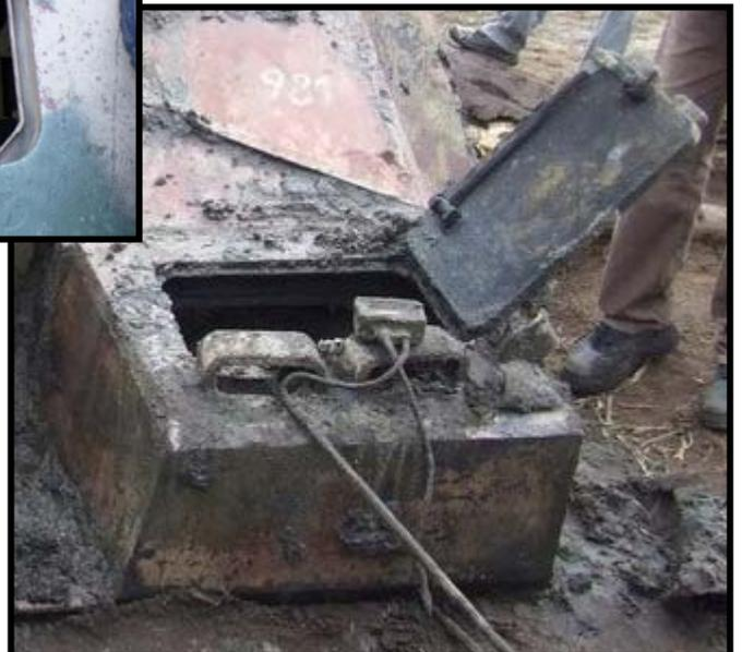
There were rain shields added to some of the periscope armored covers. These are shown in several of the extra photos in the separate files. These shields were authorized for retro-fitting by units in the field, but are not evident in all of the photos of late StuG IV's.
