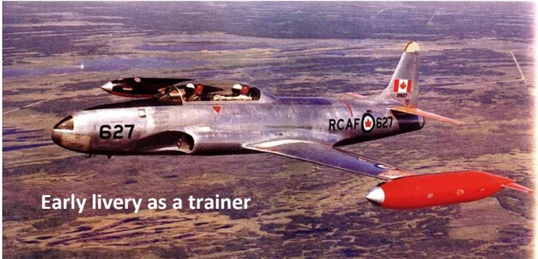
The appearance of the CT-133 is very distinctive due to the large fuel tanks usually carried on each wingtip. The CT-133 entered service in the RCAF
