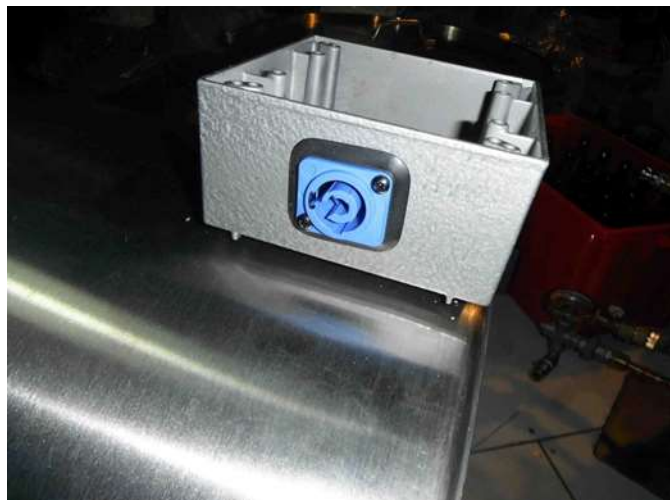
Powercon 20A socket fitted to 2400w element box:
