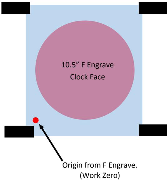
Since the stock piece is 11.25" wide and the clock face image is 10.50", that means there should be a .375" space to the left and right of the clock face. Make your work zero point .375" to the right of your stock's left edge and up far enough that you will avoid clamps and not go off the top edge of the wood. This will be your WORK ZERO for all future operations until it's cutout. Send the clock face carve.
