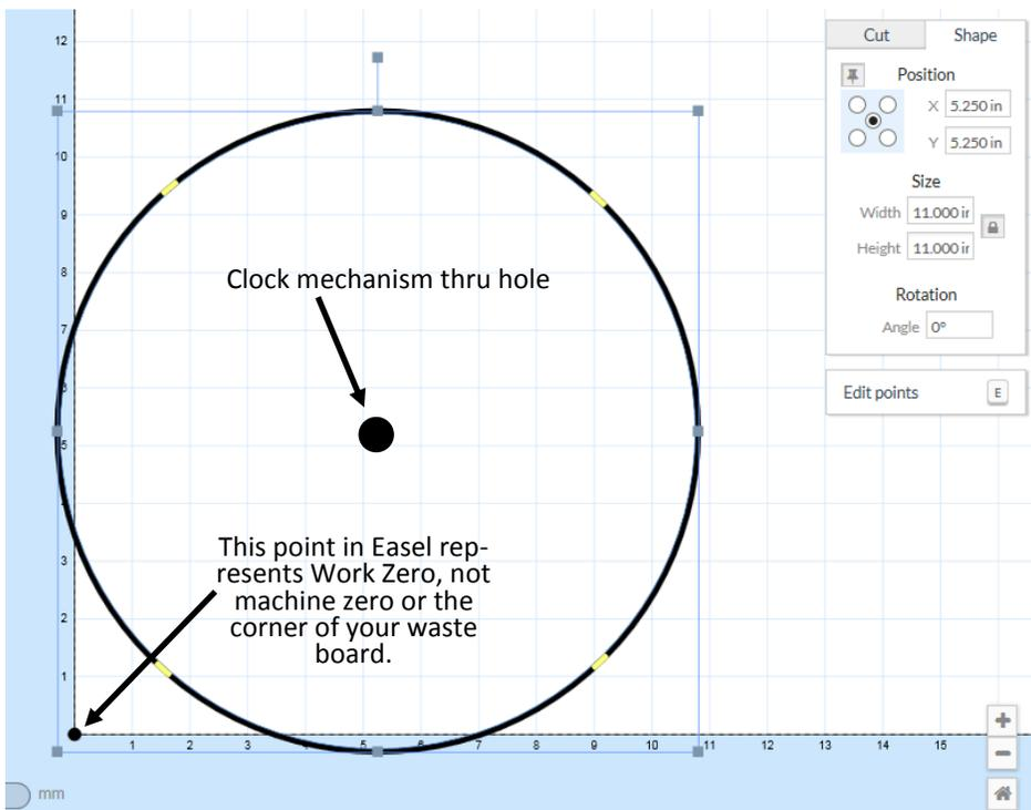
So keeping our original zero point by using the last X and Y home positions, our 11" circle is centered on the 10.5 inch clock face. It only looks like it's cutting off the grid, it's not cutting off your material because the work zero point is .375" in from the edge. Don't forget to also cut a thru hole for the clock shaft to stick thru. I use that point to center my bit on when I have to flip it over to mill a pocket for the mechanism to sit in.
