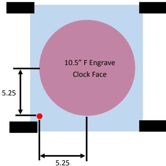
Because the clock face is 10.5" in diameter, its center is 5.25" up and over from the WORK ZERO point. Use this information to set up the circle cutout and center hole for the clock mechanism. That means you will draw a circle 11.00" in diameter with its center point at X = 5.25, Y = 5.25.
