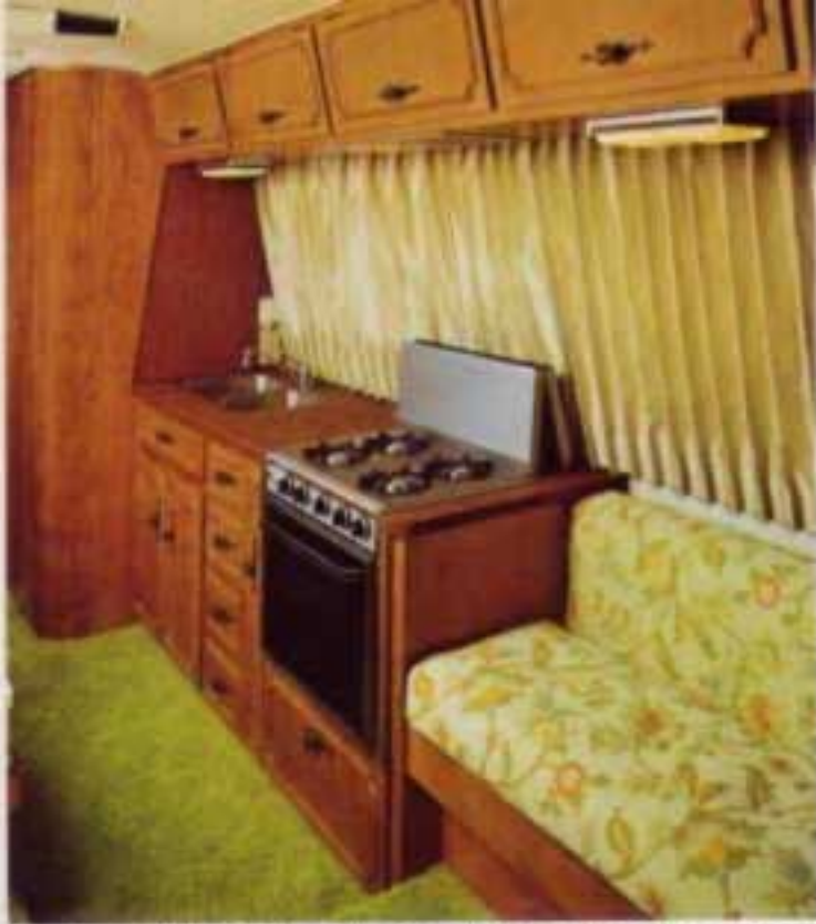
Galley has steel double sink, combination gas/electric refrigerator with freezer compartment, plus 4-burner gas range with full-size oven and broiler.
