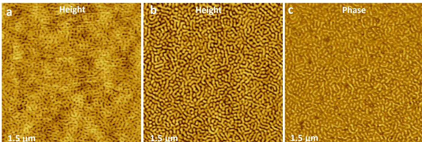
**Figure 4a-c.** Height and phase images of SBS film in AM-PI mode with Si probe ( $k = 1.93$  N/m)
