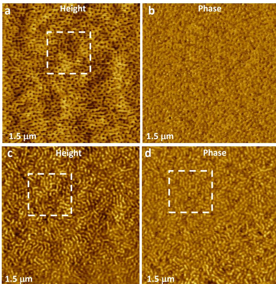
**Figure 6a-d.** Height and phase images of SBS film in AM-PI mode with Si probe ( $k = 23$  N/m) and  $A_0 = 24$  nm.
