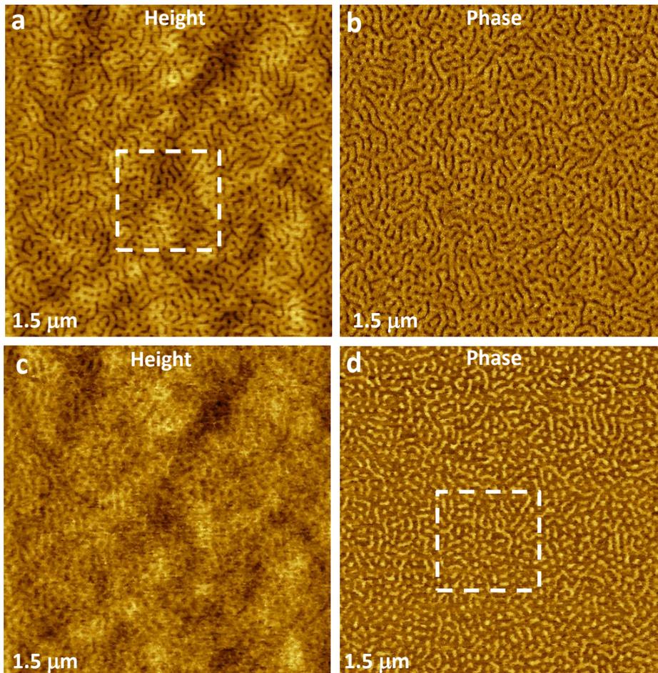
**Figure 5a-d.** Height and phase images of SBS film in AM-PI mode with Si probe ( $k = 23 \text{ N/m}$ ) and  $A_0 = 6 \text{ nm}$ .
