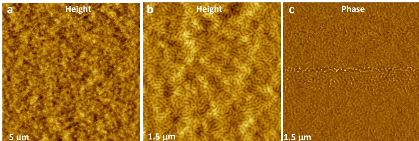
**Figure 3a-c.** Height and phase images of SBS film in AM-PI mode with Si probe ( $k = 0.065$  N/m)
