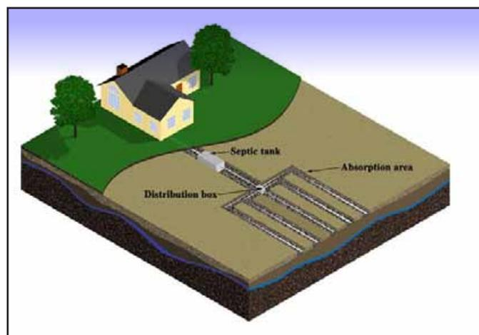
**Figure 1.** The basic design of an onsite sewage treatment system
