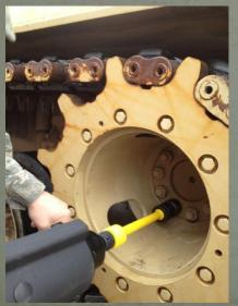
Please note that when tightening each sprocket nut, a "torque-limiting" extension was used to ensure the proper torque ( + or – 10 %).
