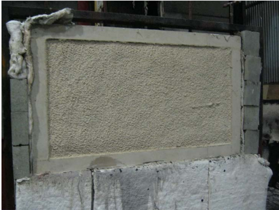
Test #2 - Exposed Side Prior to the Fire Test (Spay Applied Cementitious Fire Proofing)
