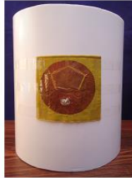
Figure 4. Photograph of the fabricated wearable antenna bent along y-plane on PVC pipe [14]. [reproduced courtesy of the Electromagnetics Academy].
